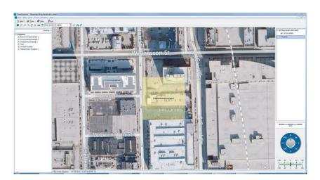
The SE-GIS module provides the geographic information system (GIS) for the StrataExplorer base application. It is used as the primary display and selection interface for the base application. Without the SE-GIS module the application will display of list of projects only and not display basemaps.
