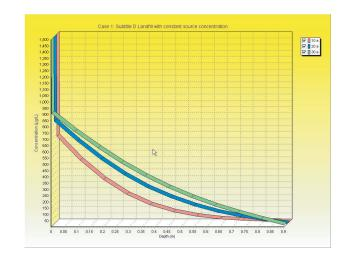
The POLLUTEv7 program provides fast, accurate, and comprehensive contaminant migration analysis capabilities. This program implements a one and a half dimensional solution to the advection-dispersion equation. Unlike finite element and finite difference formulations, POLLUTEv7 does not require a time-marching procedure, and thus involves relatively little computational effort while also avoiding the numerical problems of alternate approaches.
